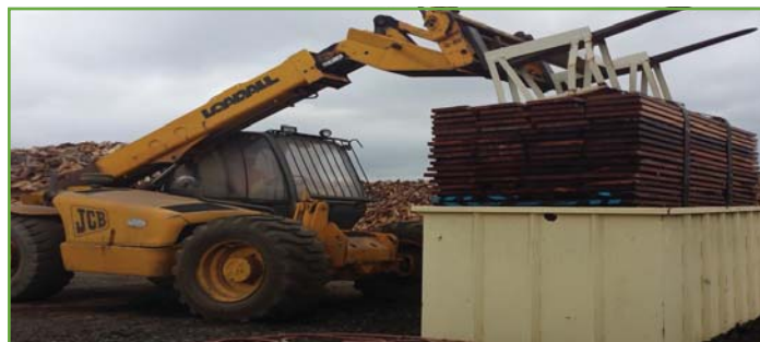
Crews do a Borax dip to deter Powder Post Beetles Used with permission by West Coast Arborists, Inc.
